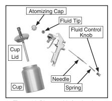
Figure 14. Disassembly for cleaning.
